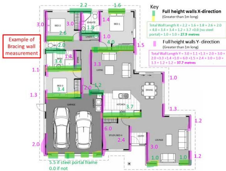
HouseCheck assumes that all walls are of the bracing material selected. This may not be the case for your house. If you know which are bracing walls and which are not you can reduce your bracing wall length to match.
